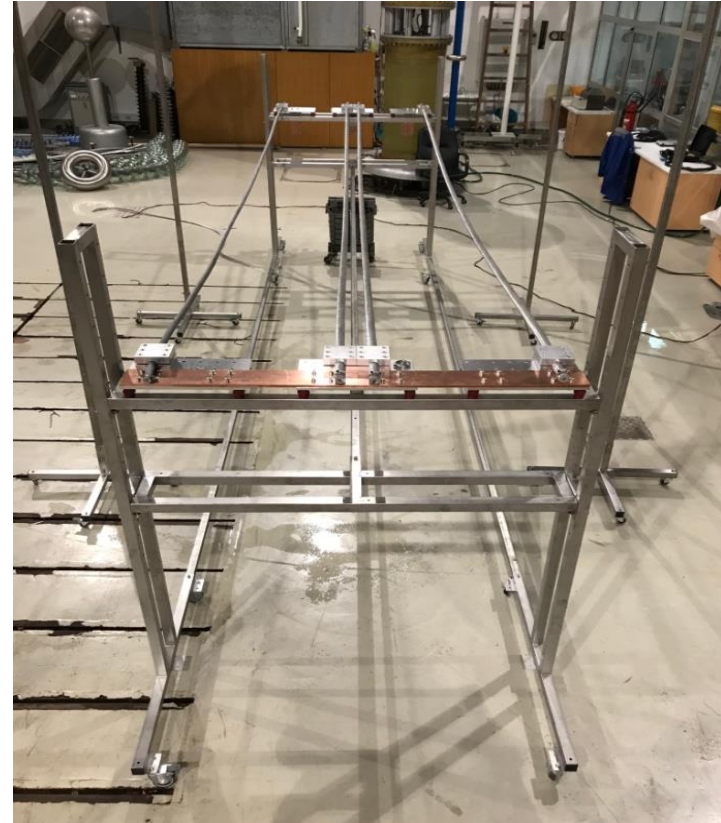
Experimental setup for measurements of conductor temperature
